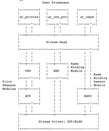
The first application illustrated (at\_printer) shows the configuration for communicating with a network print server. Note that the ATP module must be pushed before the PAP module. While it is possible to reverse the pushing order, unpredictable
